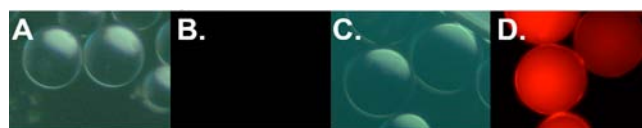
Figure 2. Fluorescent microscopic images of protein immobilization using an OPA derivative. (A) Bright-field image of resin coupled with OPA derivative. (B) Fluorescent image of resin coupled with OPA derivative. (C) Bright-field image of resin coupled with OPA derivative after conjugated with RFP. (D) Fluorescent image of resin coupled with OPA derivative after conjugated with RFP.
